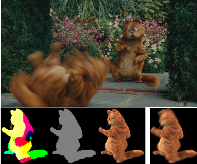
Figure 1: top: A 2k frame motion-blurred with Pixmotor was generated in under a minute on a 2 GHz dual Opteron. bottom: Pixmotor’s motion, depth, color inputs, and output.
